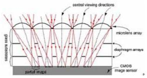
crosstalk, adjacent optical channels need to be optically isolated. In eCley, an aperture array is included in the optical system to absorb stray light.
