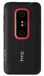
The Evo 3G was unveiled at CTIA in March. It features an autostereoscopic 540 x 960, 4.3-inch display, using a switchable parallax barrier design, we believe. There is a 1.3mpixel front-facing camera and dual 5mpixel back-facing cameras to capture 2D or 3D stills and video. It is a little unclear if the 3D video is captured in 720p or 1080p, but if it operates like the LG Optimus, 3D capture is at 720p/30.
